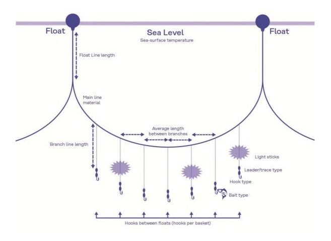
Longline (Gear Configuration): Average branch line length (meters): straight length in meters between snap and hook.
