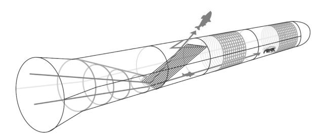
Schematic illustration of a size and species selective trawl. Entering fish are led towards the trawl floor and grid via a leading funnel. Larger fish are then led out of the trawl by the grid while smaller fish and Norway lobster pass through the grid and enter the codend. The full square mesh codend enhances escapement of small fish and undersized Norway lobster. The square mesh codend shown in the diagram is required only in Skagerrak and Kattegat.
