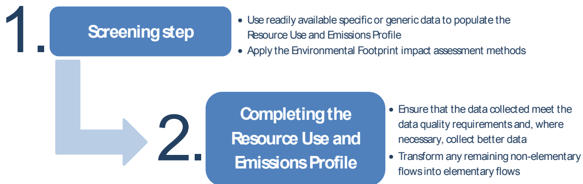
Figure 3: Two-step procedure to compile the Resource Use and Emissions Profile (the screening step is highly recommended, but not mandatory).
