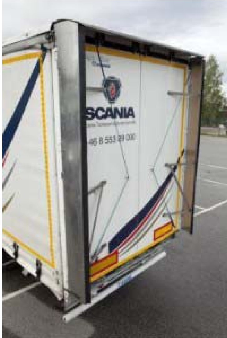
Figure 3: 500 mm deflector under test
