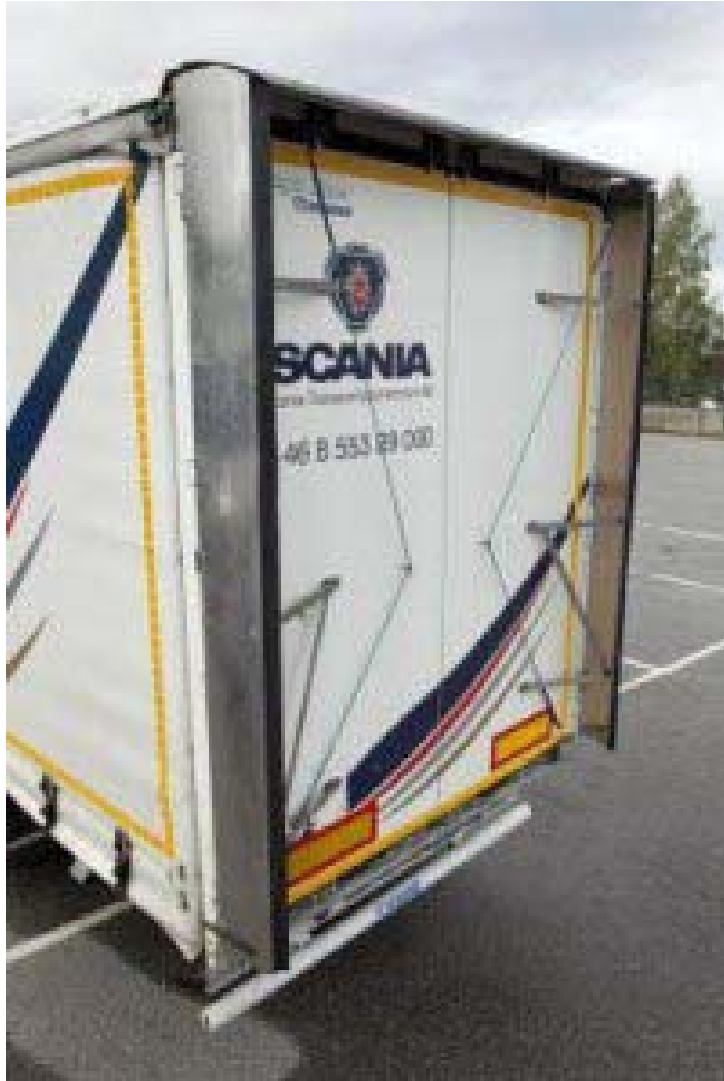
Figure 3: 500 mm deflector under test
