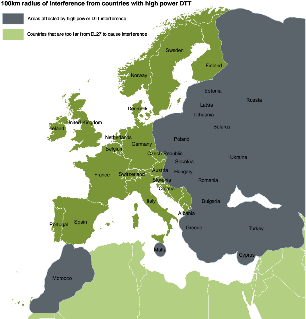
Figure: Assumption of regions in which harmful interference is caused by Member States using the 790–862MHz sub-band for high-power DTT [Source: Analysys Mason, DotEcon, Hogan & Hartson, 2009]
