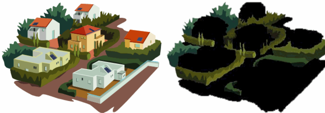
Figure 2: Visualisation of the terms 'settlement area' and 'soil sealing' 40 (source: Prokop et al, 2011).
