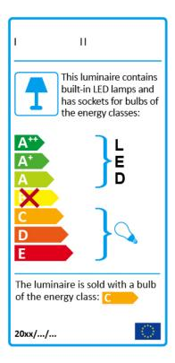
(d) Luminaire containing both non-replaceable LED modules and sockets for user-replaceable lamps, with lamps not included:
