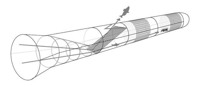
Schematic illustration of a size and species selective trawl. Entering fish are led towards the trawl floor and grid via a leading funnel. Larger fish are then led out of the trawl by the grid while smaller fish and Norway lobster pass through the grid and enter the codend. The full square mesh codend enhances escapement of small fish and undersized Norway lobster. The square mesh codend shown in the diagram is required only in the Skagerrak and Kattegat.
