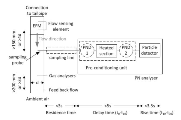
The PN analyser shall be connected to the sampling point via a sampling probe which extracts a sample from the centreline of the tailpipe tube. As specified in point 3.5 of Appendix 1, if particles are not diluted at the tailpipe, the sampling line shall be heated to a minimum temperature of 373 K (100  $^{\circ}$ C) until the point of first dilution of the PN analyser or the particle detector of the analyser. The residence time in the sampling line shall be less than 3 s.
