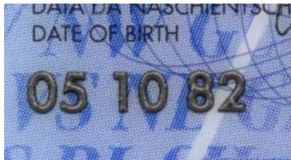
Tactile laser engraving of the date of birth
