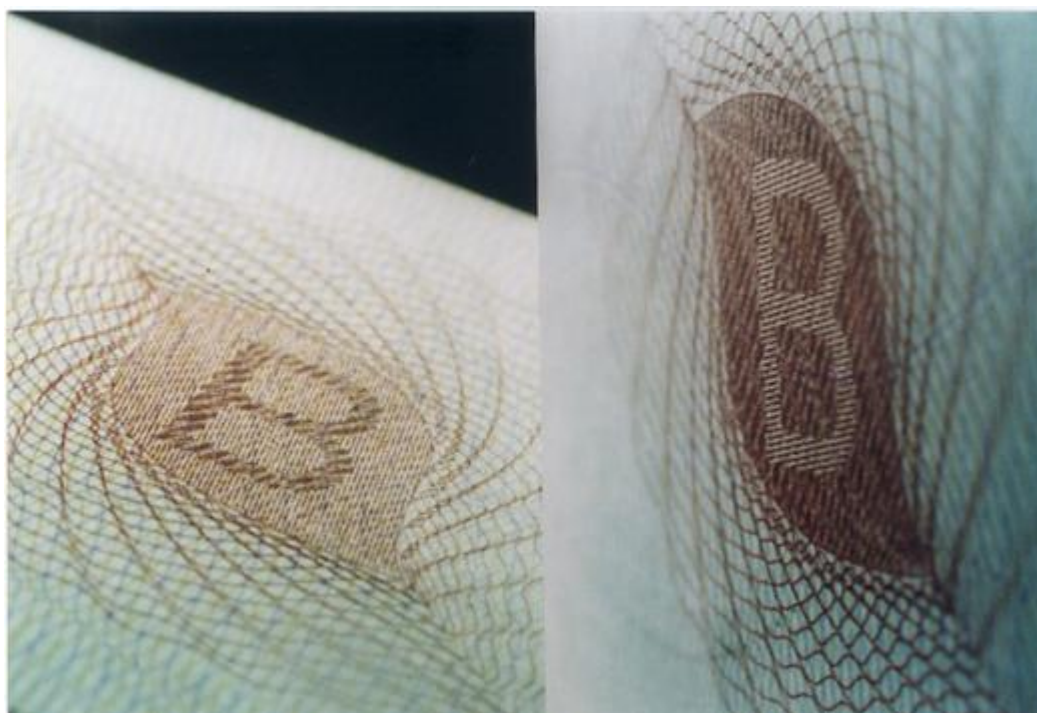
Latent image revealed by tilting the document page
