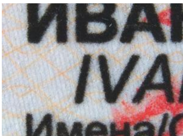
Biodata & photo integration technique: laser printing
