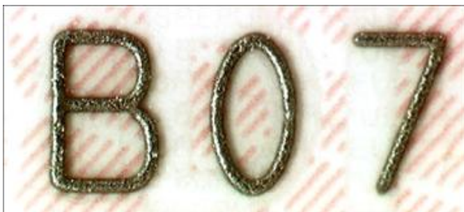
Tactile laser engraving of the numbering
