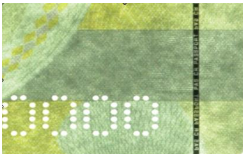
Security thread with negative microprint (by transmitted light)
