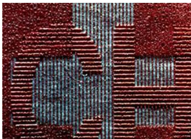
Line structure (90°) of the latent image
