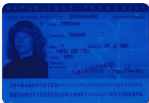
➔ Genuine document: ➔ Substrate without optical brightener
