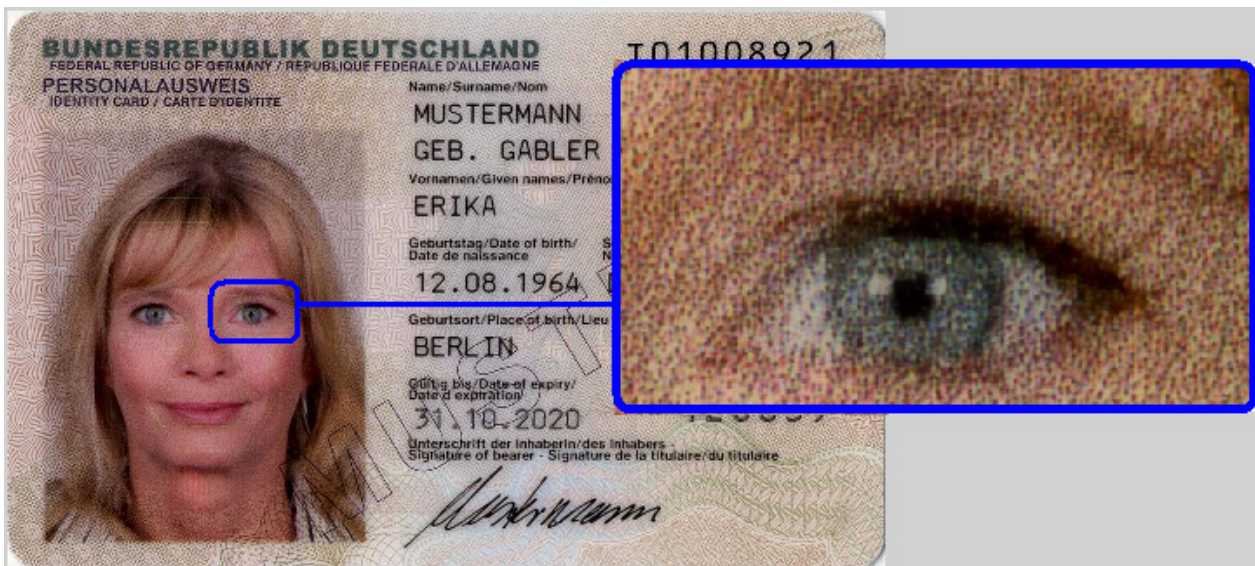
Photo integration within the polycarbonate card (Innosec Fusion® process)
