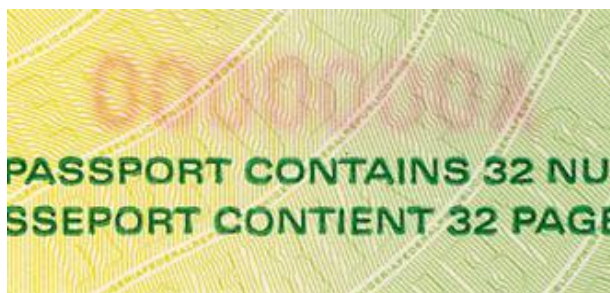
Part of the numbering ink has bled through the paper substrate and can be seen on the reverse side.
