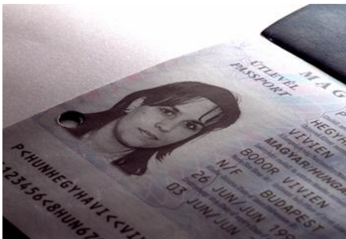
Laser-engraved integrated image
