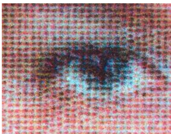
Biodata & photo integration technique: laser printing
