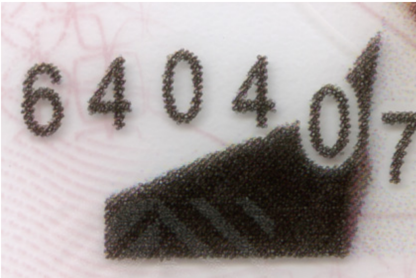
Poland: driving licence - PCP (Polycarbonate Colour Personalisation) technology
