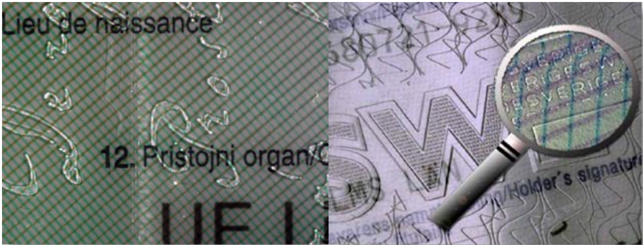
Laminate embossing with microprint
