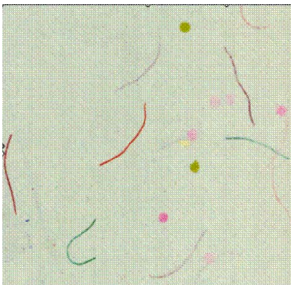
Coloured planchettes and fibres
