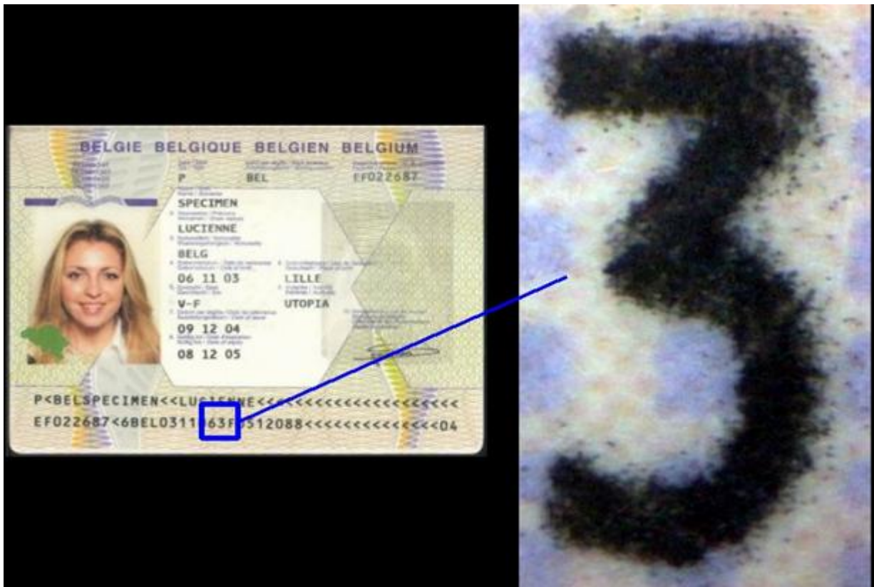
MRZ - integration technique: laser printing
