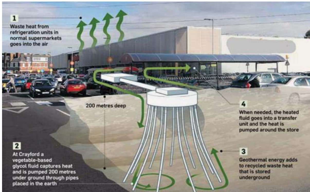
Figure 6-9. Schematic of a closed loop geothermal heating and cooling system at a UK retail store
