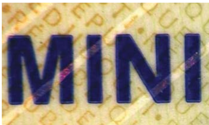
Flexo printing on → laminate
