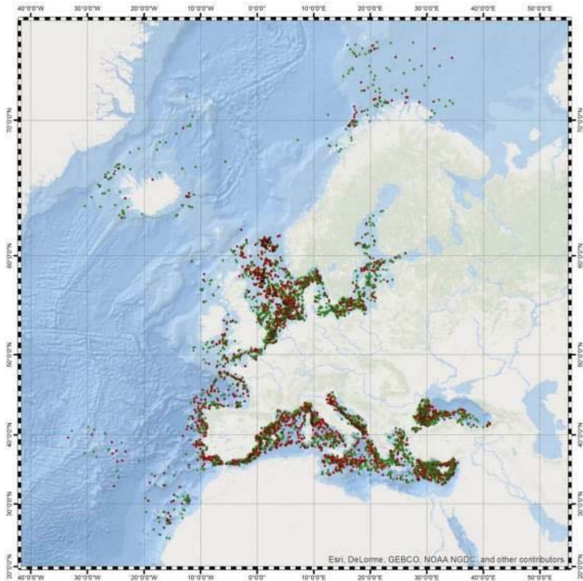
Figure 3: CleanSeaNet 2014–2016: Class A (red): “most probably oil” and Class B (green): “possibly oil or chemical product” detections in EU coastal State waters (except French Outermost Regions), Iceland, Norway, Turkey and Montenegro
