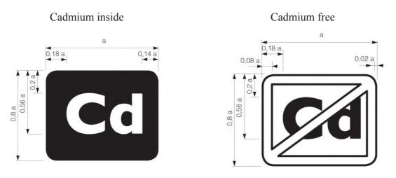
The dimension of "a" shall be greater than 9 mm and the typeface to be used is 'Gill Sans'.
