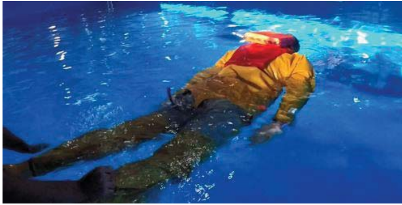
Figure 2: Test subject wearing heavy weather clothing during failure of the righting tests
