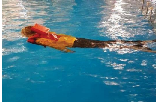
Figure 5: MSC.81(70) righting test once the ankles of the test subject have been released
