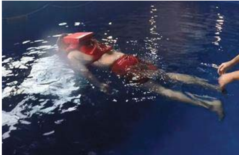
Figure 1: Typical MSC.81(70) righting test once the ankles of the test subject have been released
