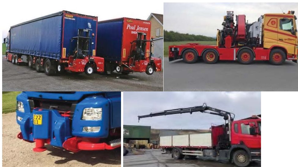
Figure 9. Illustrations of typical vehicles included in the segment (truck mounted forklift, foldable cranes and support legs).
