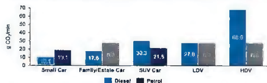
Figure 5: The average of CO 2 emitted, by fuel and vehicle type, whilst idling for one minute
