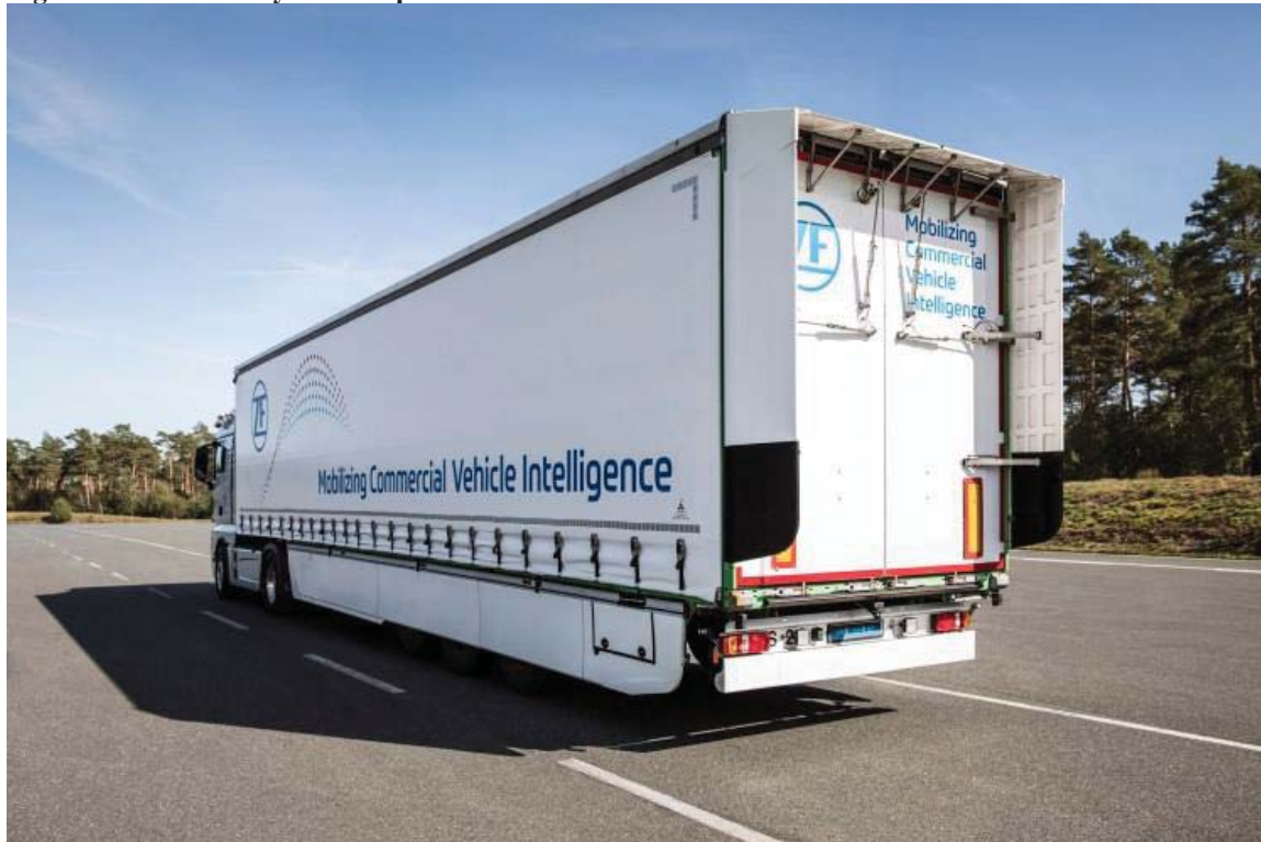
Figure 17: Rear aerodynamic flaps on a semitrailer
