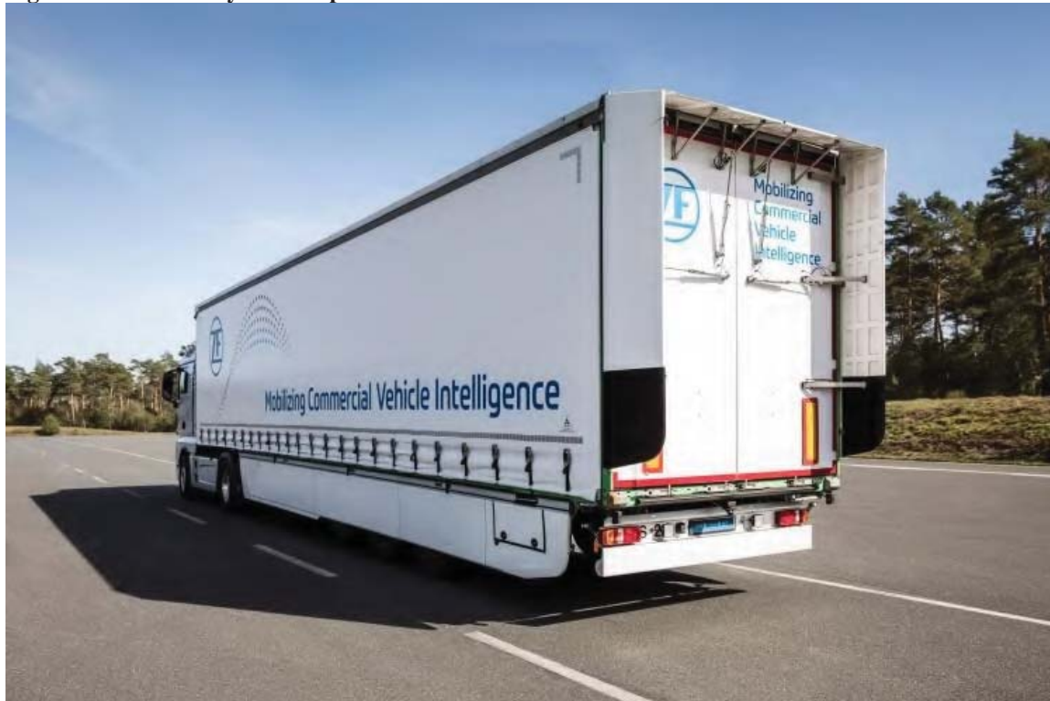
Figure 17: Rear aerodynamic flaps on a semitrailer
