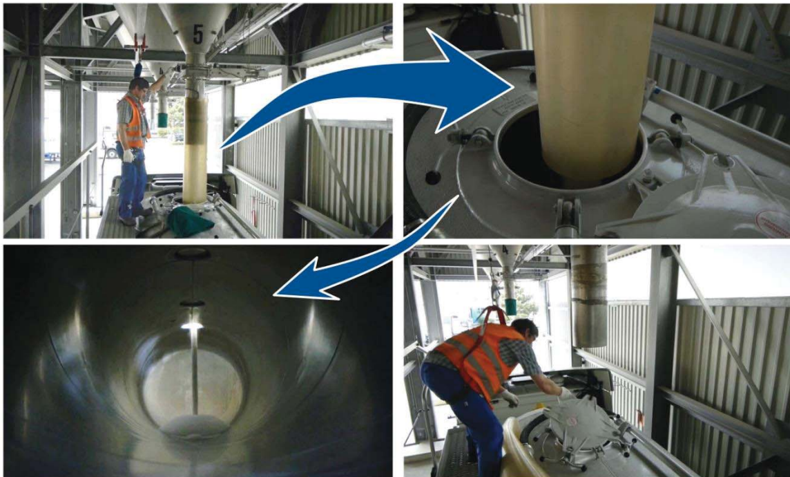
Figure 12: Loading pellets into a silo truck
