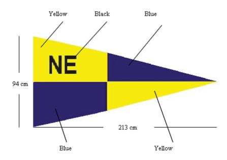
Boarding crafts shall display one inspection pennant as indicated below. The pennant may be half scale. The pennant may be painted on the hull or any vertical sides of the craft. When
