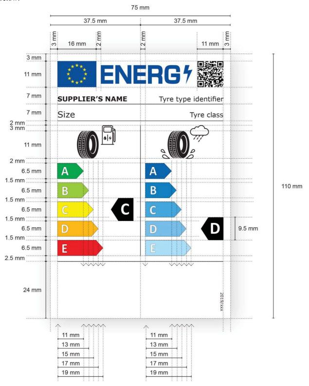
2.1.1 Label design for the bottom part of the label for all tyres other than tyres which satisfy the minimum snow index values set out in UNECE Regulation 117, or the relevant minimum ice index values, or both.
