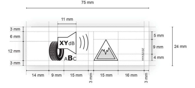
2.1.4 Label design for the bottom part of the label for tyres which satisfy both the relevant minimum snow index values set out in UNECE Regulation 117 and the minimum ice index values.
