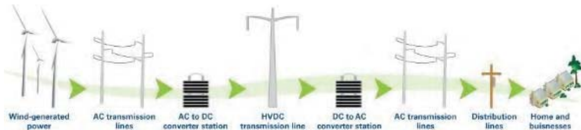
Figure 157 HVDC system integrated in the AC grid
