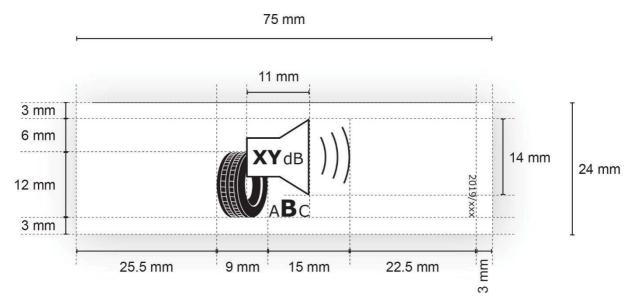
2.1.2 Label design for the bottom part of the label for tyres which satisfy the minimum snow index values set out in UNECE Regulation 117.
