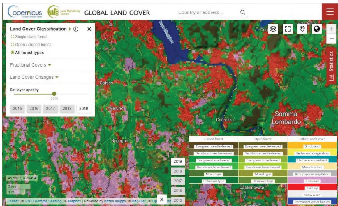
Figure 22 - Copernicus annual global land cover product: this global 100m resolution map product, derived from PROBA-V satellite observations, is processed to ensure continuity with Copernicus Sentinel-2 observations.
