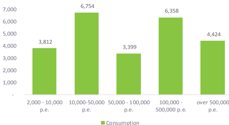
Figure 41 Energy consumption in GWh per year, estimates per WWTP-size in EU. Source: adapted from Ganora et al. (2019).
