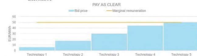
Figure 8: Illustration of the current electricity wholesale pricing method and a possible alternative
