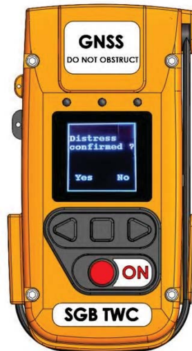
Figure 2: Mechanical design of SGB TWC beacon prototype with display
