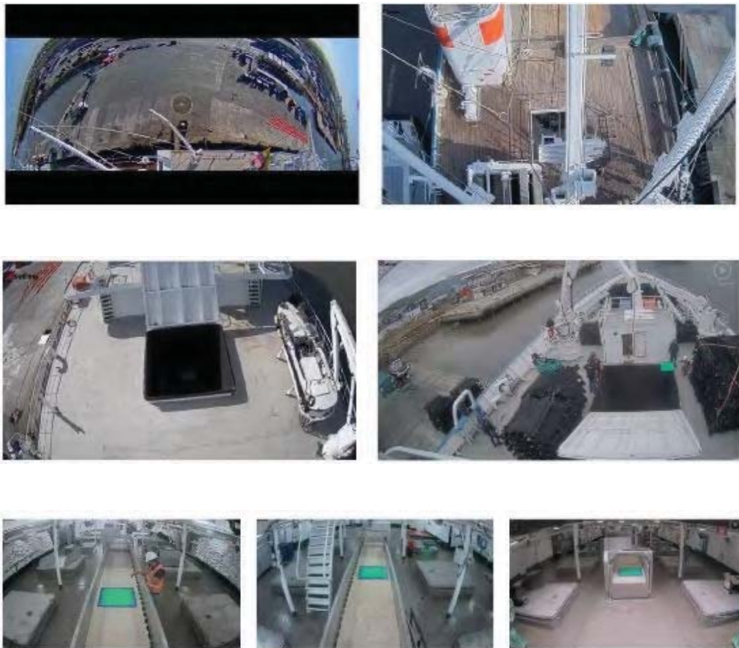
Figure 1. (A) An example of a 6-cameras EM system installed in a purse seiner covering main areas of fishing and fish handling operations (from Murua et al., 2020b) and (B) 7-cameras EM system (4 in the upper deck and 3 in the well deck) installed in a purse seine covering main areas of fishing and fishing handling operations including 1 more camera in the conveyor belt: (B1) 360° Panoramic view camera (e.g port side view), (B2) Crows nest stern view camera, (B3) Working deck crane camera view , (B4) Foredeck view camera, (B5) Conveyor belt stern camera view, (B6) Conveyor belt middle camera, and (B7) Conveyor belt bow camera (source: Digital Observer Services).
