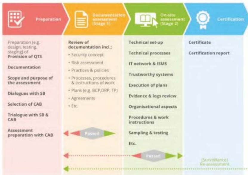
Figure 3. Typical conformity assessment (certification) process flow 9
